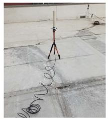
Figure 1: The Harsh/Synergetics 14A-N omnidirectional antenna mounted on a tripod.
